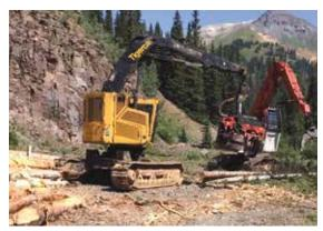
Above Highway 550, a timber loader and a logging processor turn felled trees into lumber. Photo: Alex Shelley
